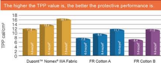
All tested fabric is washed with domestic washing method Use NFPA heat source according to the method suggested by ASTM-D4108
